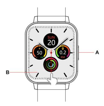
Button A: Long press to switch ON/OFF, short press to turn ON/OFF the screen.
