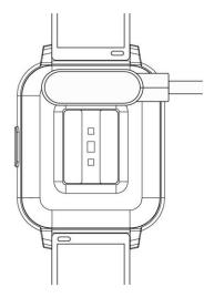
\* Please note that the two contacts of the charging cable cannot contact the conductor at the same time, which will cause the circuit to burn.
